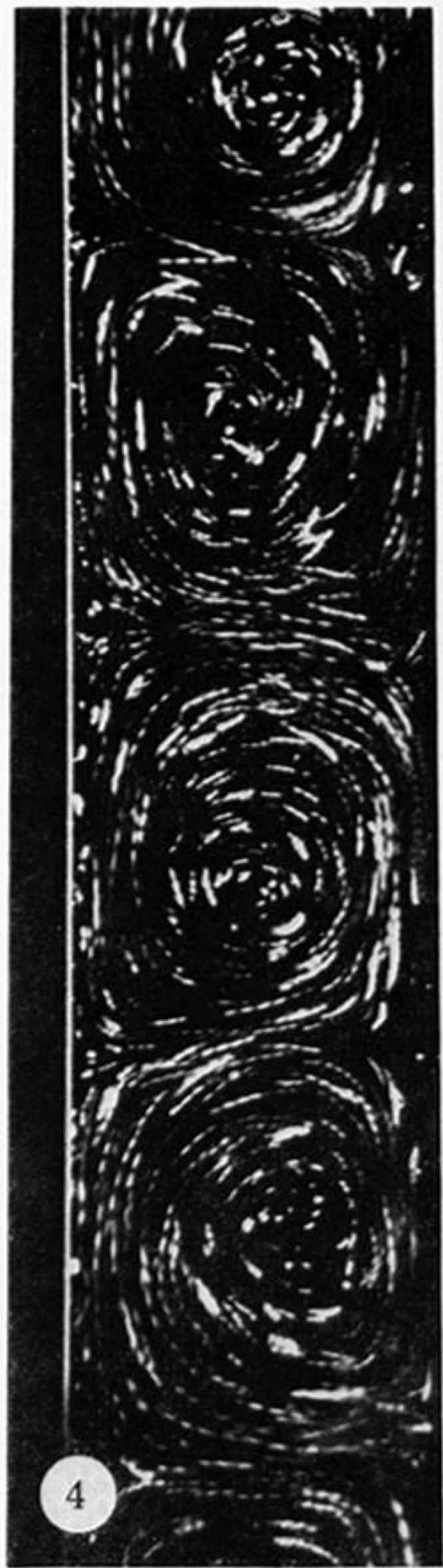
FIGURE 4. Sectional view of Taylor vortices illuminated by a planar radial light beam. (Gap between cylinders, 1 cm.)
